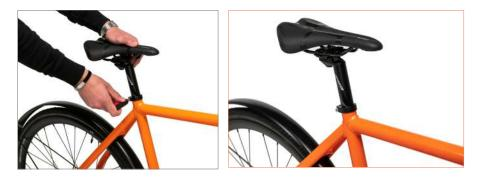
• To install the seatpost start by loosen the bolt found on the seatpost collar using a 4 mm allen wrench, apply a small quantity of bike grease on the bottom of seatpost. It should easily slide into the frame. Make sure to slide the seatpost past the minimum insert line; align your saddle to the desired height.
