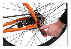
Before each ride, please check the correct tension of the **belt** or the **chain**; both need to be properly placed in location for the correct use.
