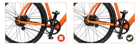
Verify that all bolts, fasteners of front and rear wheels, and kickstand (if any) are steady. Check that both **pedals** are properly tightened in the crank arms; if needed remove and reinstall the pedals, following the instructions in **Chapter 6.**
