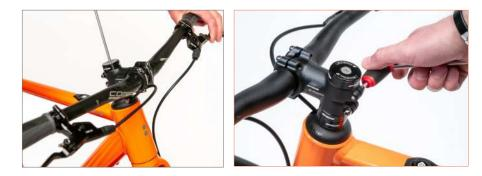
• First step, align the handlebar with the front wheel. Slightly tighten the bolt of the cover on the fork steerer with a **4 mm hexagonal allen key**, until you encounter no play in the headset or any jamming. In case the movement of the handlebar is not fluid enough, slightly loosen the bolt.
